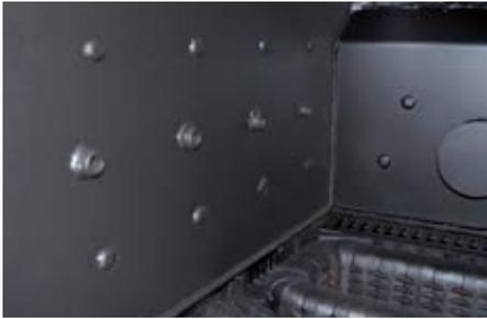
*Post combustion air inlet holes*
